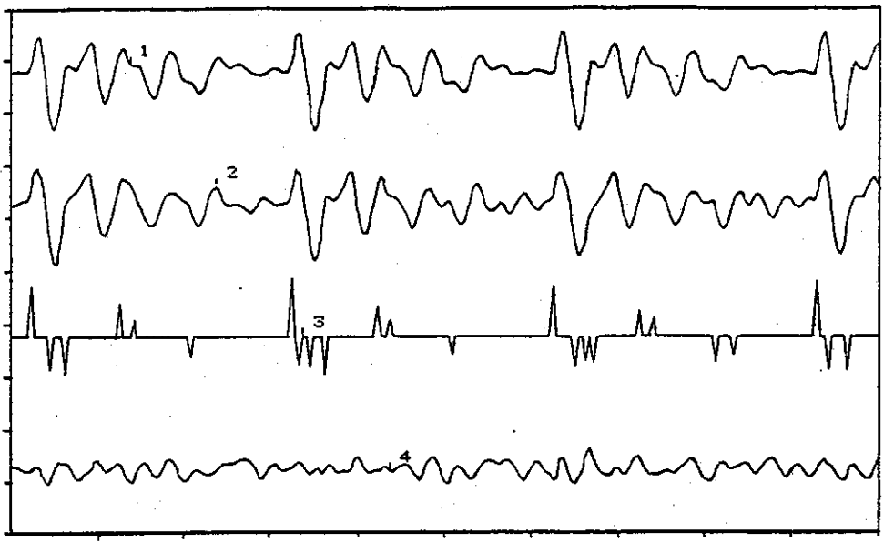
PLOT #1 : ORIGINAL SPEECH SIGNAL PLOT #2 : SYNTHETIC SPEECH SIGNAL PLOT #3 : EXCITATION SIGNAL PLOT #4 : ERROR SIGNAL
