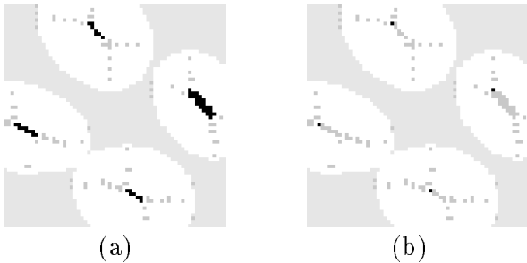
Figure 1: (a) Skeleton and Ultimate Erosions of a portion of the image “Coffee Grains”. The Ultimate Erosions are the black Skeleton points. (b) A subset of the Ultimate Erosions (the four black points). Their quench values, in addition to the position of all the Skeleton points, are sufficient for perfect reconstruction.
