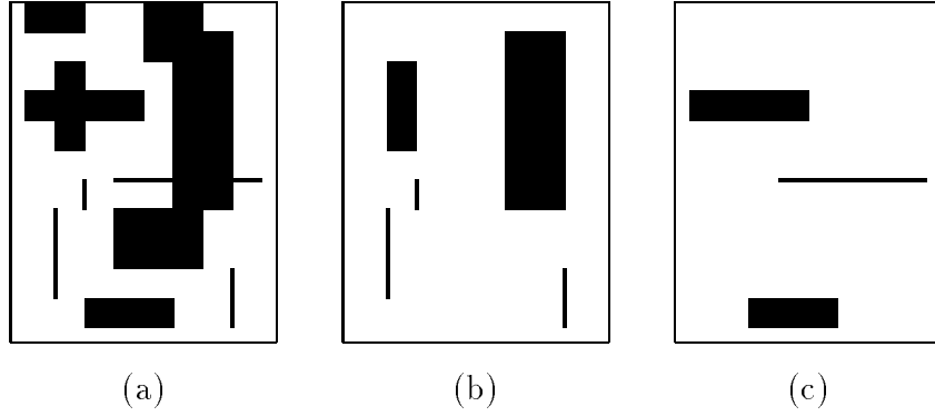
Figure 5.1: Shape Classification via an MSES: (a) An image composed of rectangular features. (b) Features for which C_1 \geq 75\% . (c) Features for which C_2 \geq 75\% .
