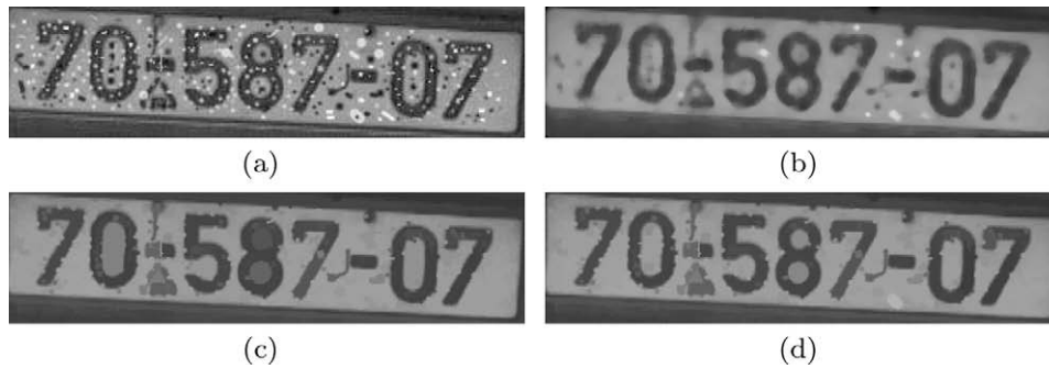
Fig. 8. (a) Input image, artificially corrupted, (b) filtered with a median filter, (c) filtered with regular “quasi-self-dual” opening by reconstruction, and (d) filtered by the EWT-based opening by reconstruction, using circle SE of radius 4.
