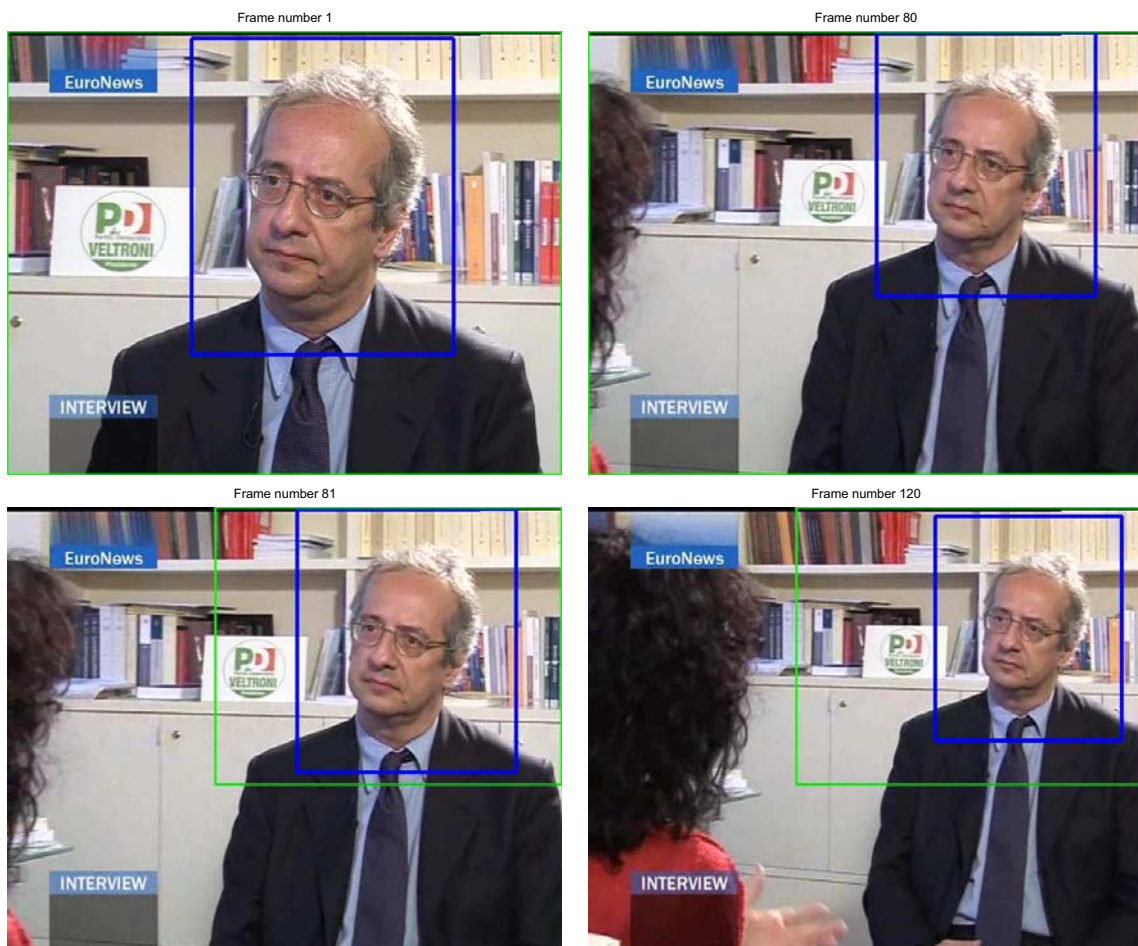
Figure 6.2: Frames from the movie “Euro News Zoom-Out” - with the ROI marked as a blue rectangle and the ROD marked as a green rectangle. The ROD always contains the ROI.
