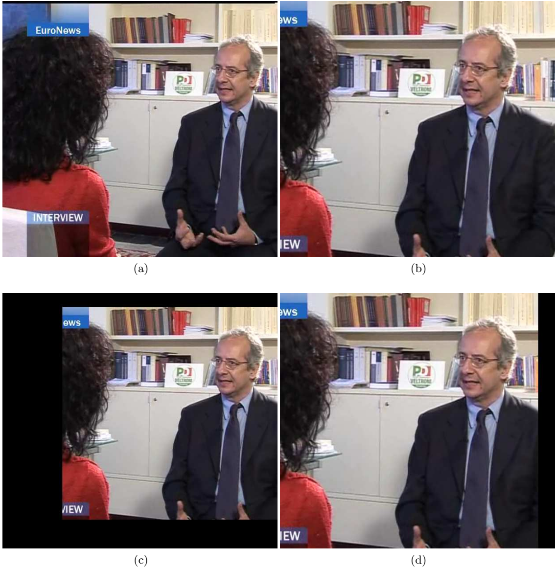
Figure 3.13: Example of reducing fixed-size display effects. Image (a) is the previous frame. Image (b) is the current frame which is a scaled and shifted version of the previous frame. Image (c) is the previous frame after zeroing out the parts that do not appear in the current frame. Image (d) is the current frame after zeroing out the parts that do not appear in the previous frame.
