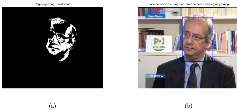
Figure 8.5: Region growing result. (a) Combination of region growing on the skin-color detector output and region growing on the frame using an AND operation. (b) Face region is marked on the frame.
