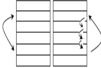
Figure 4.1: Illustration of random perturbations for the Binary Switching Algorithm. Left: "switch" ; Right: "move"
