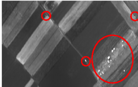
Figure 5.1: 30th band of a hyperspectral image cube with anomalies marked in white and encircled by red ellipses.
