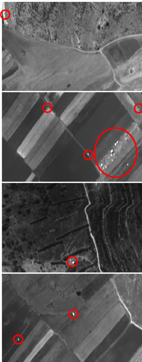
Figure 4.4: Ground truth. A 30th-band of each one of 4 image cubes used for evaluation. The ground-truth anomalies were manually identified, marked in white and encircled in red.
