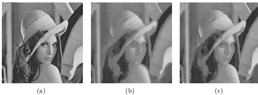
Figure 3. (a) Original image, (b) EWT erosion by square SE 5 \times 5 , (c) EWT opening by square SE 5 \times 5 .
