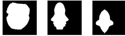
Fig. 8. 3 projections, from left to right, on xy , xz and yz , respectively, of a mirrored face. The xy projection was excluded from our face recognition scheme due to its high similarity between different faces.
