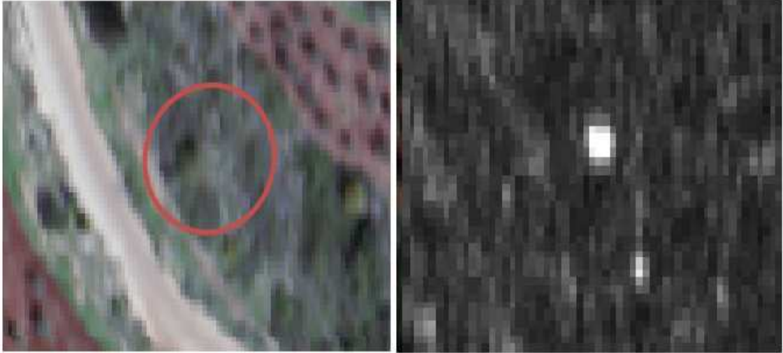
Figure 2.4: A typical RX false alarm. Right image - RX score map with a strong false alarm , Left image - An RGB representation of the area with the false alarm marked by a red ellipse
