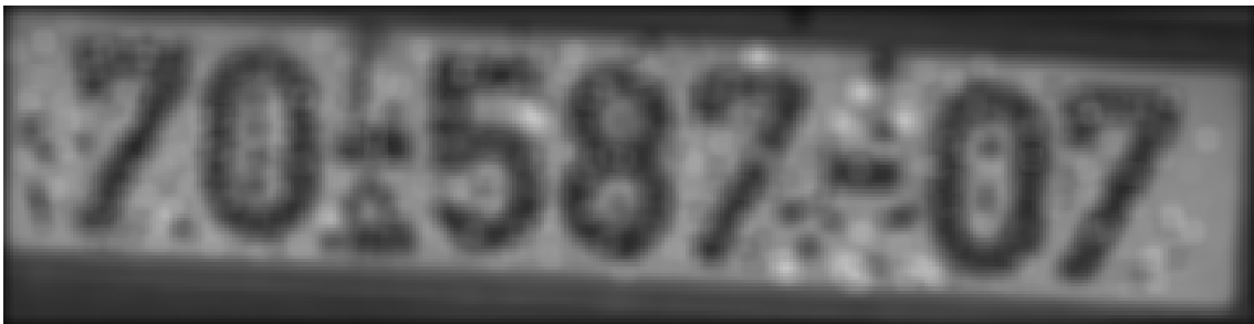
Figure 6.33: License plate image filtered with an averaging filter.
