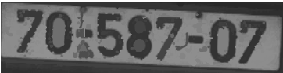
Figure 6.36: License plate image filtered with regular self dual opening by reconstruction.
