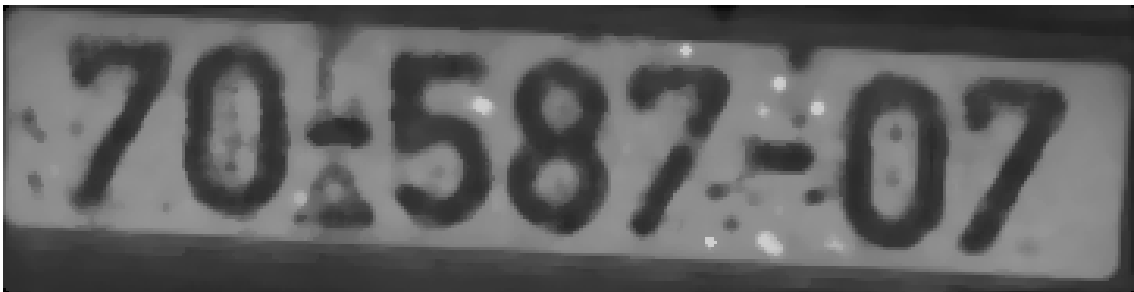
Figure 6.34: License plate image filtered with a median filter.
