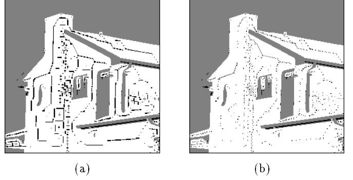
Fig. 2: (a) A binary image and its skeleton, using a 3 \times 3 squared structuring-element, (b) a reduced skeleton obtained by the proposed algorithm.
