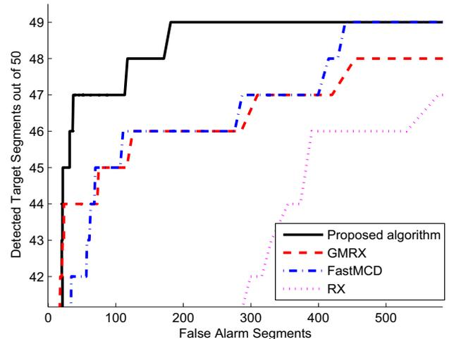
**Fig. 5.** ROC curves corresponding to RX, GMRX, FastMCD and proposed algorithm
