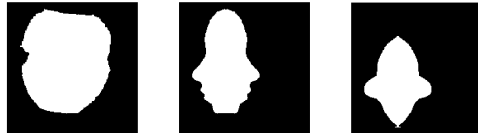
Fig. 8. 3 projections, from left to right, on xy , xz and yz , respectively, of a mirrored face. The xy projection was excluded from our face recognition scheme due to its high similarity between different faces.
