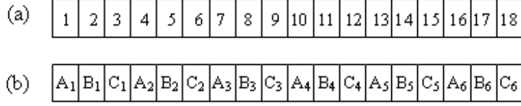
Fig.8: (a) Long window types – coefficients arranged in ascending order: 1-18. (b) Short window type – interleaving the coefficients of the 3 short MDCT transforms: A-C, according to their ascending order: 1-6.
