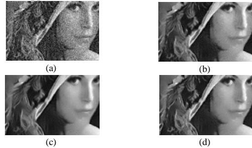
Fig. 6: Denoising variations of the image Lena (256x256) with \sigma_n = 20 , a zoom-in view of the shoulder and face (flat regions) and of the feathers (texture). (a) Noisy image. (b) Denoised image using conventional NLM with a Box dissimilarity kernel. (c) Denoised image using conventional NLM with a Uniform dissimilarity kernel. (d) Denoised image using proposed approach.
